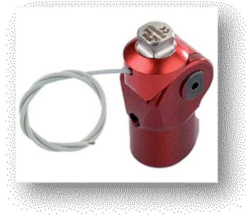
These knees are often referred to as 'stance control' knees and contain a weight-activated friction brake that stops the knee from bending. These knees swing freely, like a door hinge, when there is minimal or no weight put on the prosthesis. The knee locks once weight is applied. If the amputee attempts to put weight on the prosthesis when the prosthesis is partially bent, the weight-activated friction brake prevents the prosthesis from buckling.
