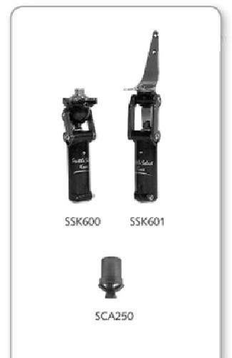
which allows the amputee to walk at various speeds. When the amputee increases in walking speed, with cylinder limits the amount of air and allows the knee to bend more quickly. When the amputee decreases walking speed, with cylinder increases the air content, making the knee bend more slowly. The prosthetic knee is locked at heel strike and is automatically unlocked during toe-off.
