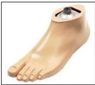
Dynamic elastic response feet flex at heel strike and midstance and then spring back at late stance. This imitates the energy return characteristics of a normal ankle, which reduces energy expenditure and improves gait
